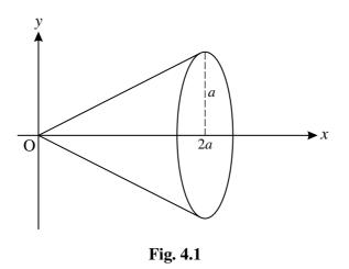
(i) Show, by integration, that the moment of inertia of the cone about its axis of symmetry is  $\frac{3}{10}Ma^2$ . [You may assume the standard formula for the moment of inertia of a uniform circular disc about its axis of symmetry and the formula  $V = \frac{1}{3}\pi r^2 h$  for the volume of a cone.] [8]
